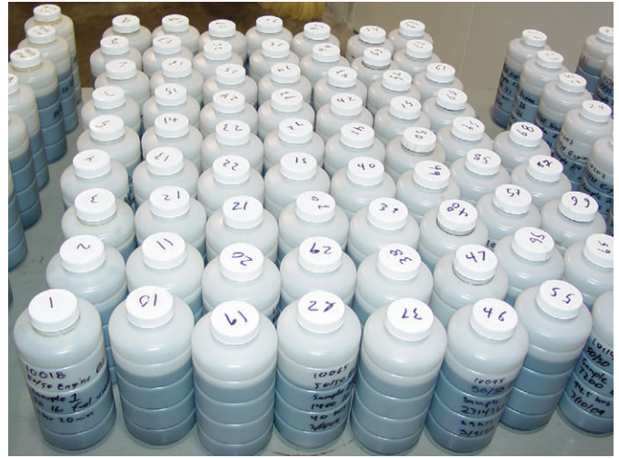
Samples of biobased engine oils taken from diesel engine tests at the UNI-NABL Center.
