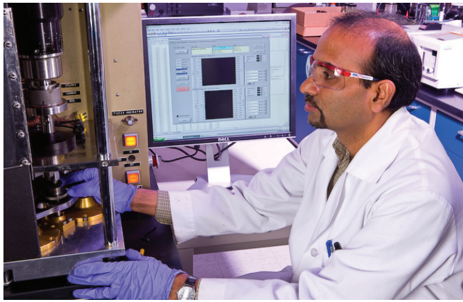
Dr. Brajendra Sharma, senior research associate at Penn State University, uses a standard four-ball test method to measure friction and wear properties of vegetable oil-based lubricants.
